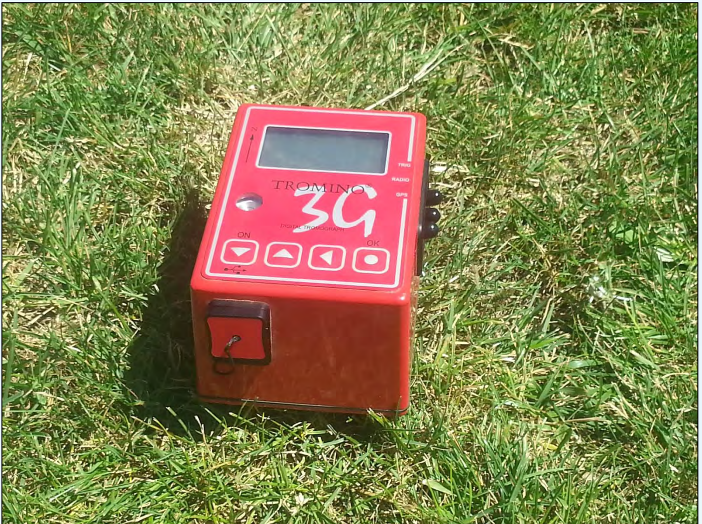
Image: Passive seismic instrument used to measure seismic waves as they arrive from a wide range of natural and artificial sources. (Courtesy Sarah Buckerfield)
