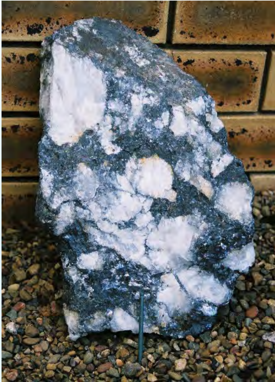
Breccia from the Fitzpatrick orebody, North Broken Hill Mine, NSW. Image courtesy J.R. Lord.
