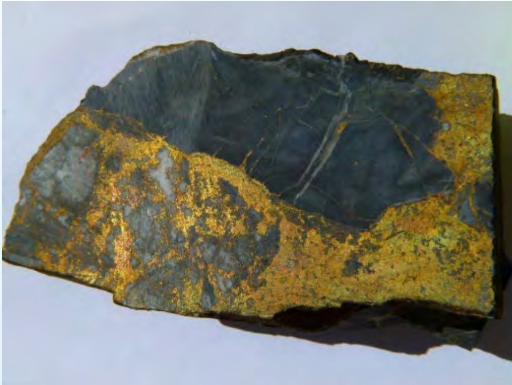
Medium grey carbonaceous chert with fracture fill chalcopyrite and silica (white). WG Perkins specimen. Image courtesy J.R. Lord.
