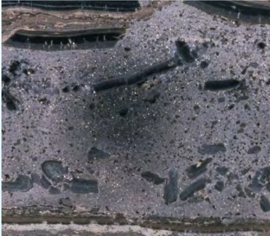
Galena remobilised between black shale beds and brecciating the thinner ones between them; MICAf 6910N & 2830 RL. Image courtesy W.G. Perkins.
