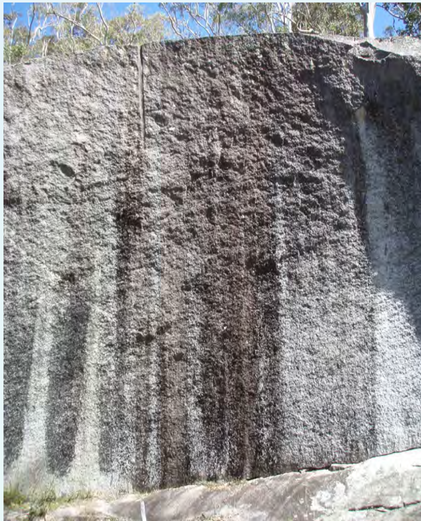
Face of the Louttit Quarry in 2012. Note lack of jointing and drill hole at the centre top. Face about 6 to 7 m high. Image courtesy B. Pillans.
