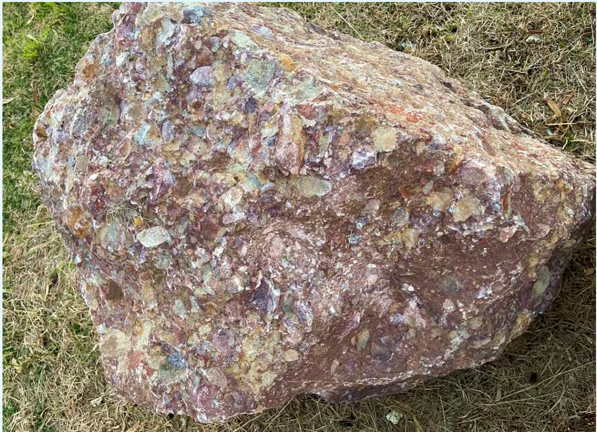
Owen conglomerate boulder showing the typical white quartzite clasts in a red sandstone matrix. Field of view is about 1.2 m. Image courtesy R. Bottrill.
