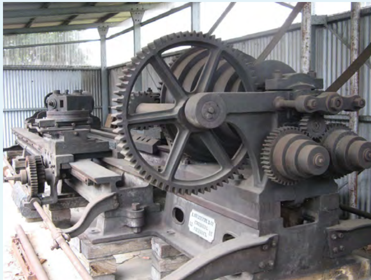
Abernethy stonemason's lathe used for making granite column sections, Moruya Museum. Image courtesy K. McQueen.
